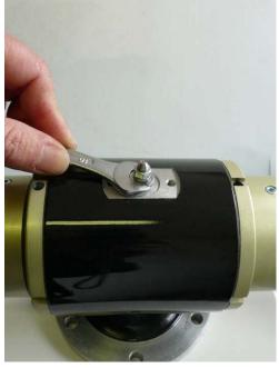
5) Secure minimum angle setting nut by tightening the locking nut using #8 wrench. At the same, hold shaped angle setting nut in place using #10 wrench.
