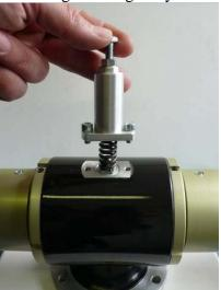
2) Remove angle setting body to gain access to rod with minimum angle setting mechanism.
