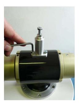
TIP: fast and precise setting of minimum angle of attack can be performed on the aircraft after installation of propeller with accessories. Procedure:
