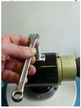
3) Secure M6 screw using M6 locking nut to keep it from turning.
