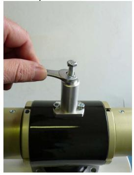
2) Set M6 screw to maximum angle of attack position.
