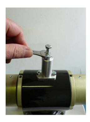
TIP: fast and precise setting of maximum angle of attack can be performed on the aircraft after installation of propeller with accessories. Procedure:
