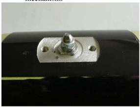
3) Loosen locking nut using #8 wrench. At the same, hold shaped angle setting nut in place using #10 wrench.
