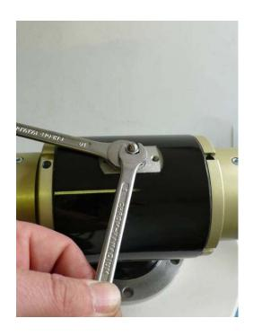
6) Replace angle setting body. Before replacing it, check its location on propeller hub – correct location is marked with centering inspection number. Use Loctite to secure socket head screws M5 and torque slightly, using no more than 4Nm.
