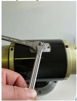
4) Set minimum blade pitch using shaped angle setting nut. Screwing out reduces the angle, screwing in increases the angle.
