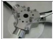
Fix the propeller hub to the base of propeller cone using the screws M8x100. Tighten the screws by tightening moment 22 Nm. (195in/lb)
